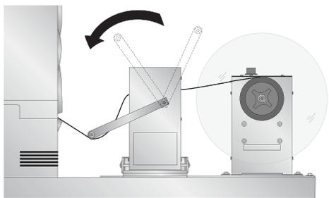
**i Important Note:** The taping process occurs very quickly so you may not get the label stock attached correctly the first time you try it. It is important to attach the label stock centered on the core. If the attached label stock is too far to the right or left the paper may fold over itself and cause an uneven wrap. If you think the label stock was not attached properly, cancel the print job using the control panel on the front of the printer.
