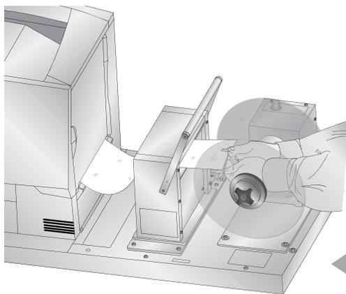
**8b** The stock will continue to feed at a slower speed. When it reaches the rewinder, attach it to the top of the empty label core. Position the stock so that it that it is centered on the core.
